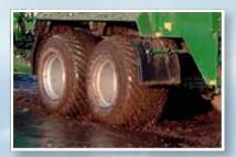
The **large-volume tyres** reduce the tractive power requirement and prevent soil compaction even under wet harvesting conditions.
