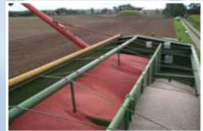
The tank volume of the transfer trailers from HAWE Wester can now be split longitudinally at the ratio of 60 / 40. The separator system of the transfer trailer tank can be fitted easily and also removed again.
