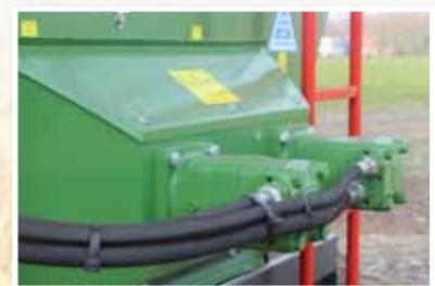
Under each of the hoppers there is a hydraulically driven auger. The filling of the seed drills is remotely radio controlled from the comfort of the tractor cab.
