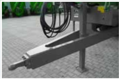
Hydraulic parking stand and mechanical drawbar suspension .
