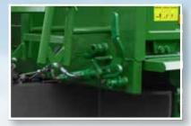
The **sidewall unlocking system** can also be hydraulically actuated as an option.
