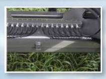
**Lubrication strip** on the axles. All lubrication points are centrally located.
