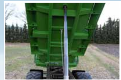
Stable trough floor on a solid frame construction.
