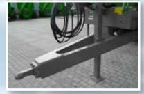
Hydraulic parking stand and mechanical drawbar suspension.
