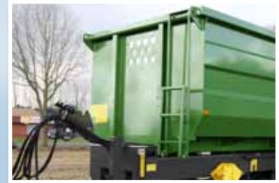
Standard ladder on the front wall.
