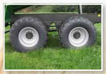
The standard equipment includes heavy running gear with **parabolic suspension**, BPW axles and generously sized brakes.
