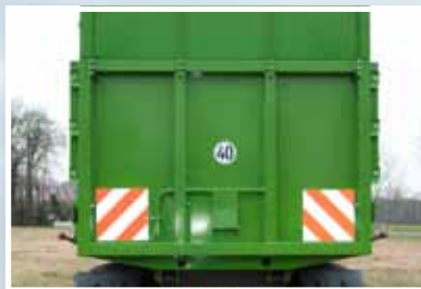
Reinforced tailgate with a solid frame made of square tubing for permanent sealing.
