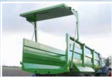
Wide opening tailgate , protected cylinder.
