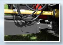
The **positive steering system** is controlled by a Bowden cable.
