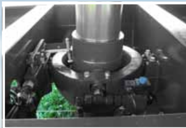
Shut-off valve and rapid lowering valve on the tipping ram.
