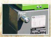
Automatic chain tensioner Visual monitoring of automatic chain tensioner.
