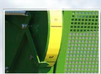
Labelling Standard tailgate opening label at the front of the forage harvester.
