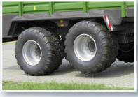
Lift axle for increased traction under difficult conditions and reduced rolling resistance during road travel.
