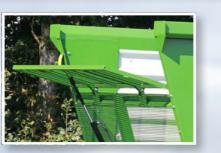
**Hydraulically folding front wall** All HAWE silage transport trailers feature a transparent front wall with a hydraulically folding upper section.
