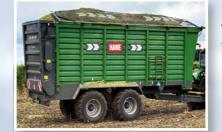
HAWE Cover Load compartment cover with hyrdaulic drive. For safe, lossless road transport. (Equipment)
