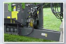
Hydraulic parking stand and hydro-pneumatic drawbar suspension.
